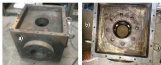
Figure 10: Constant Volume Combustion Chamber (CVCC) a) Assembly b) Top View
